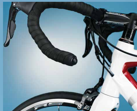
The rider controls the motor via the bar-end switch (shown in situ, right) – a discreet way of concealing the operation of the unit
